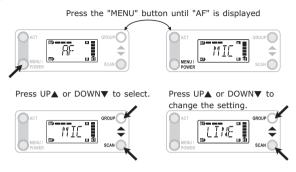
This operation provides for switching MIC or LINE.
